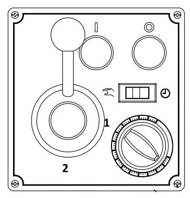
AE-35 is furnished with two button-switches, which control power to the mixer.
